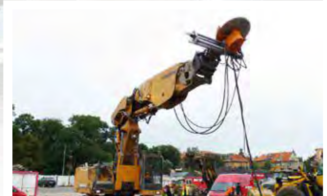
🕒 Echidna D4HS high speed rock saw with multiaxial cutting head. (Prague, Czech Republic)
