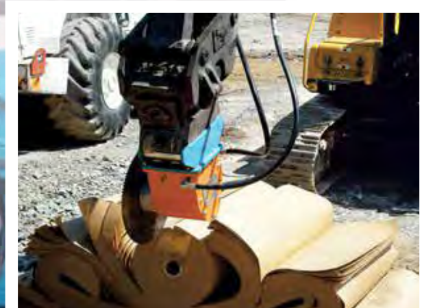
☛ Echidna rocksaw used for cutting paper rolls at a paper mill. (Visy, Australia)
