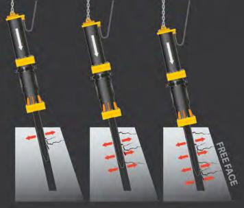
1st Step: Insert half of the total length of wedge and operate the Yamamoto splitter to split.
